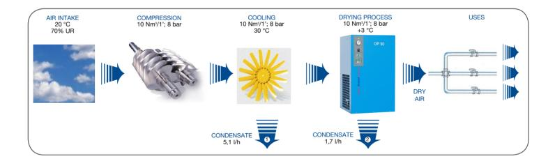
For example, 5.1 l/h of condensate is separated from a compressor with an output capacity of 10 Nm<sup>3</sup>/min and an ambient intake air temperature of 20°C and 70% relative humidity, whilst operating at a delivery pressure of 8 bar(g) and cooling the air to 30°C.
